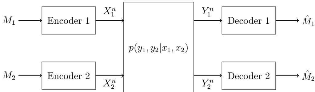
Figure 1.1: A discrete memoryless interference channel
