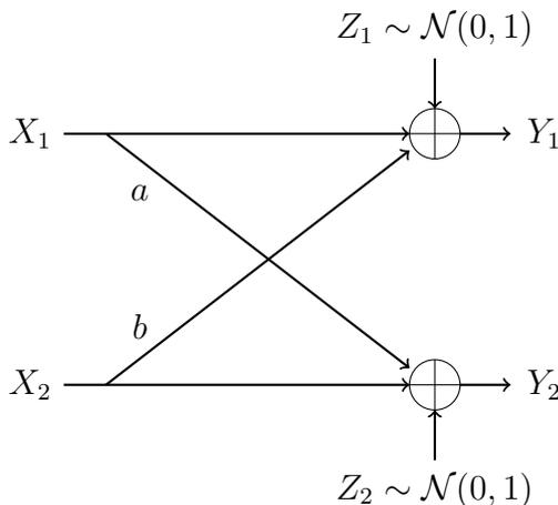
Figure 1.2: Gaussian interference channel
